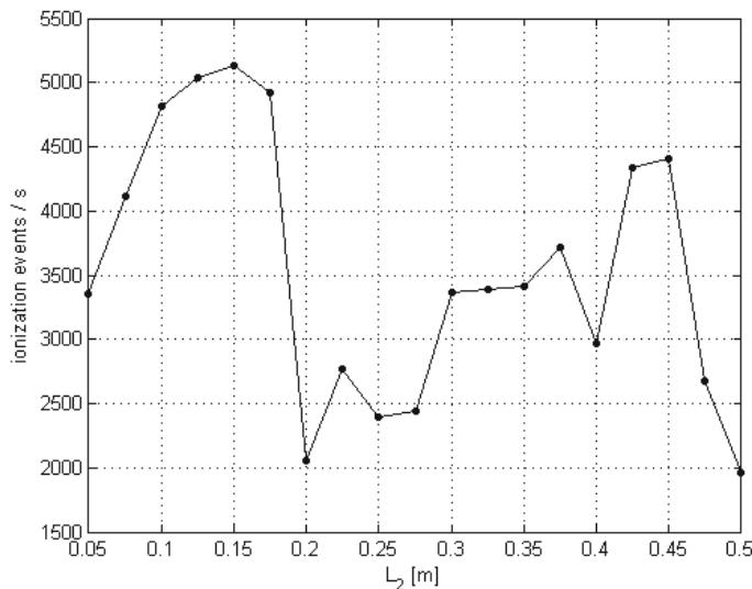
Ionization of H<sub>2</sub> background (10<sup>-8</sup> mbar), which introduces weak dissipation in the chaotic map.
