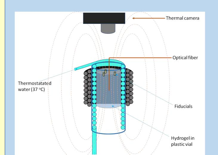
External thermalization system (liquid tube circulating system connected to a reservoir at controlled temperature) used to reach a quasi-adiabatic condition
