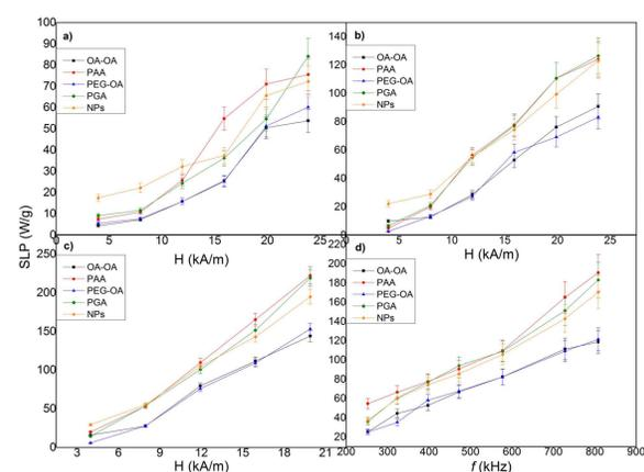
Figure 2: The SLP values for the sample with different coatings at 252 kHz (a), 397 kHz (b) and 728 kHz (c). In (d) SLP as a function of frequency at 200 Oe is shown.
