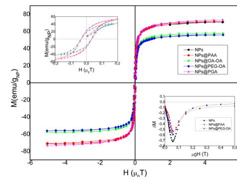
Figure 1: Hysteresis curves at 2.5 K. Top inset: zoom at low field to show hysteresis loops. Bottom inset: Henkel  $\delta m$  curves, where its clear the dominant effect of dipolar interaction.
